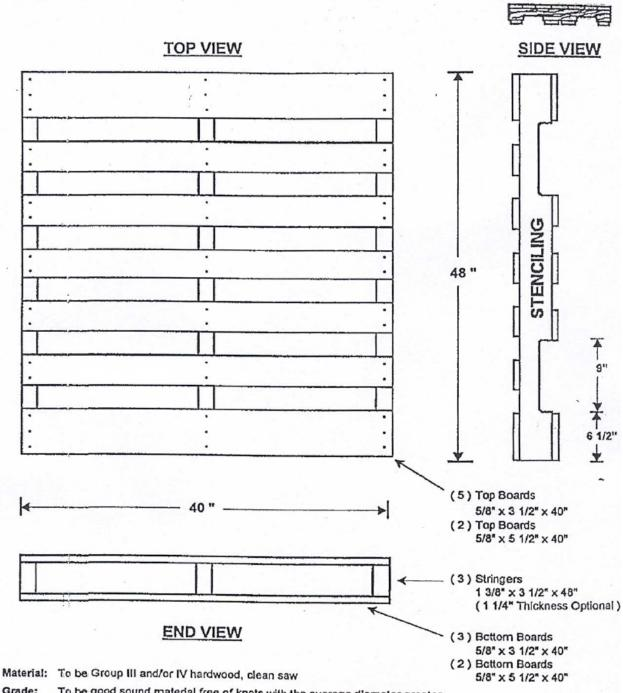
To be good sound material free of knots with the average diameter greater Grade: than one-third the width of the pieces or other defects of a more serious nature
